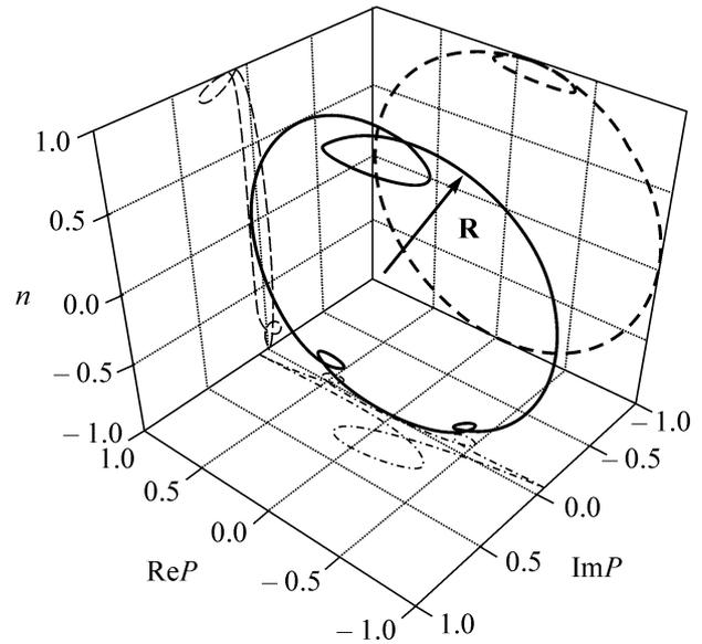
**Fig. 3.** (Solid line) Trajectory of the Bloch vector  $\mathbf{R}(x=x_0; t) = \{\operatorname{Re}P; \operatorname{Im}P; n\}$  on a unit sphere at a certain point of the medium  $x = x_0$  when the zoomeron-like pulse propagates. The dashed lines correspond to the projections of the shown trajectory on the coordinate planes. Each loop of the trajectory corresponds to one oscillation of the pulse.
