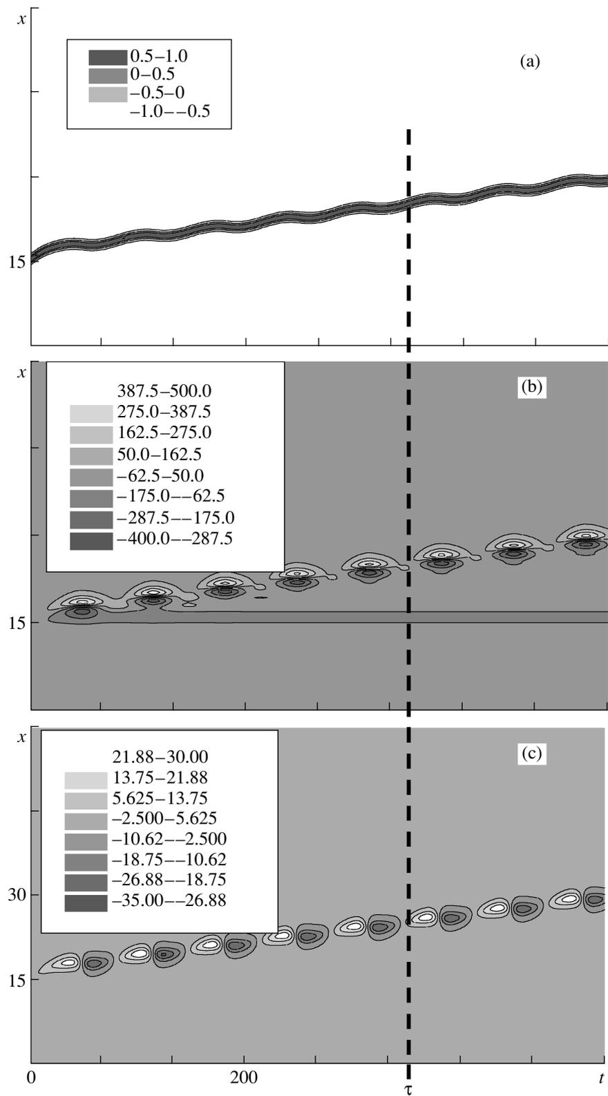
**Fig. 2.** Dynamics of the (a) inversion  $n(x, t)$ , (b) difference  $\delta\tilde{\Omega}(x, t)$  (arb. units), and (c) total  $\delta\Omega(x, t)$  (arb. units) internal-mode fields of the zoomeron-like pulse. The vertical dashed straight line corresponds to the time  $t = \tau$  at which the amplitudes of internal-mode fields are equal to zero and the velocity of the pulse is maximal.
