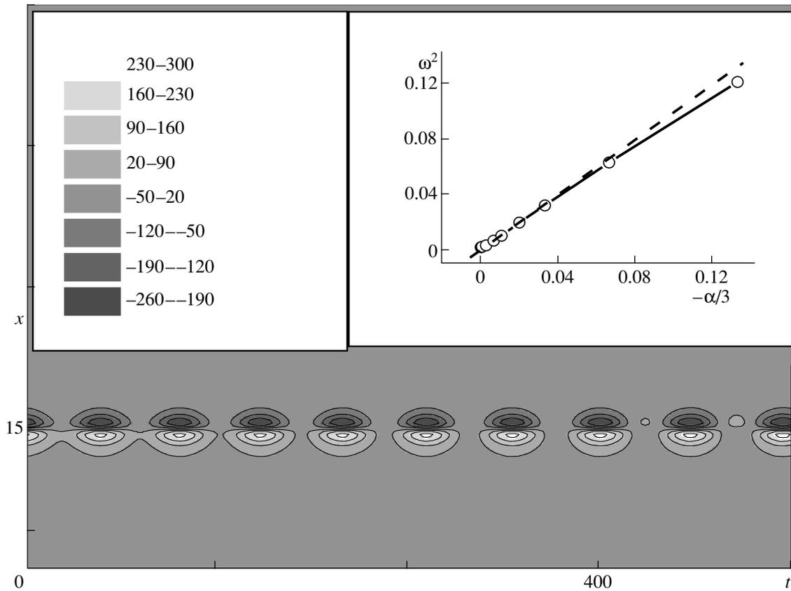
**Fig. 1.** Space–time dynamics of the difference field  $\delta\tilde{\Omega}$  of the internal modes of the Bragg soliton in the presence of beatings of two modes with nonzero and zero frequencies. The inset shows the square of internal-mode oscillation frequency  $\omega$  vs. the soliton-profile perturbation parameter  $\alpha$  (dashed line) as calculated by Eq. (9) and (solid line) as obtained by numerically integrating Eqs. (1) with initial conditions (3), (5), and (10).
