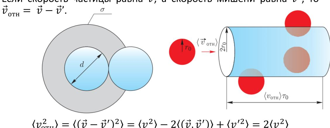
$$\langle v_{\text{OTH}}^2 \rangle = \langle (\vec{v} - \vec{v}')^2 \rangle = \langle v^2 \rangle - 2 \langle (\vec{v}, \vec{v}') \rangle + \langle v'^2 \rangle = 2 \langle v^2 \rangle$$
