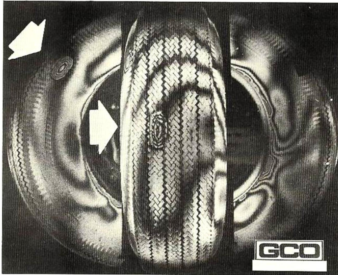
FIG. 31. Double exposure holographic interferogram of two views of a car tire showing clearly the local separation that has occurred between various plies (courtesy of G. C. O., Inc., Ann Arbor, Michigan.)
