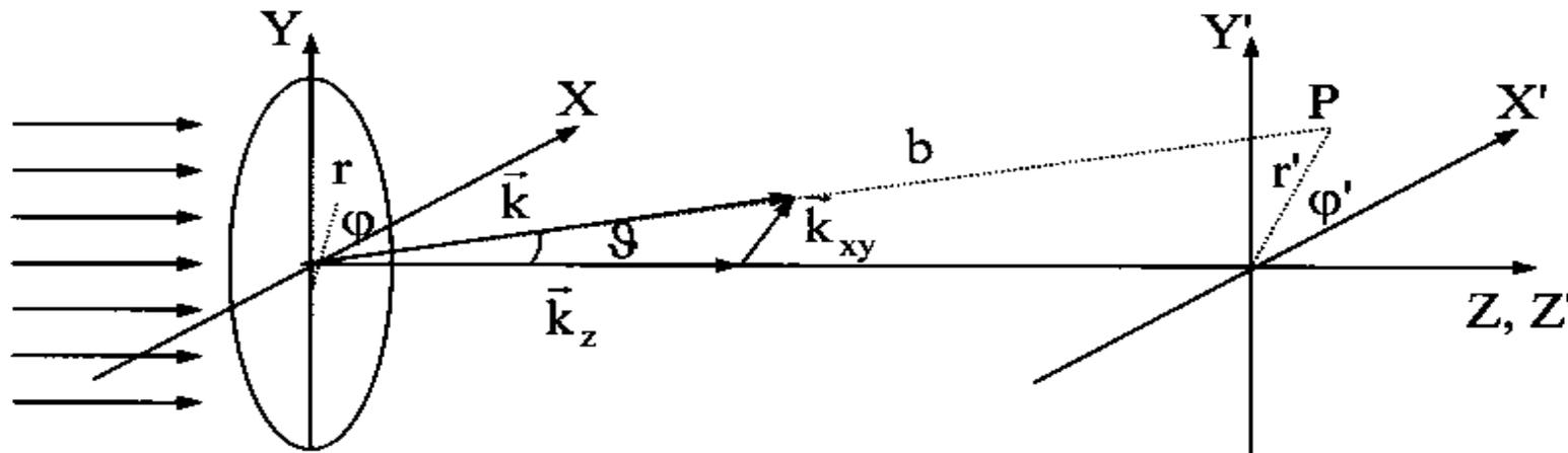
$$\sin \vartheta = \frac{r'}{b} \quad k_{xy} = k \sin \vartheta$$
